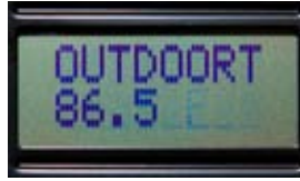
OUTDOORT - Shows temperature outside of incubator.
