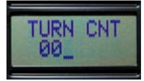
TURN CNT - Shows amount of times the turner has turned. Resets at 1000. No count on hatcher models.
