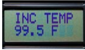
INC TEMP - Shows actual temperature inside incubator.
