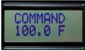
COMMAND - Shows desired set temperature.
